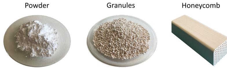
Figure 1.4.: Examined adsorbent configurations of binderless zeolite 13X. The depicted adsorbents are manufactured by Chemiewerk Bad Köstritz GmbH, Germany.
