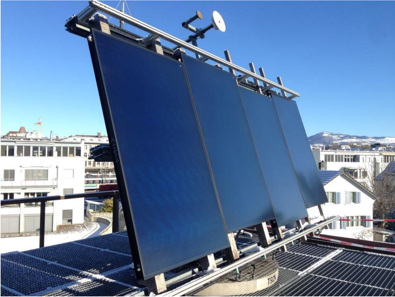
Figure 1: The four collectors on a solar tracker for pre-ageing.
