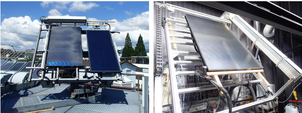
Figure 2: The collector on the outdoor test rig of one of the labs for thermal performance testing (left). Only the collector on the right side part if the RRT, the second collector is a reference collector. (right side) The collector installed on a solar simulator for different iterative tests with varying parameters.
