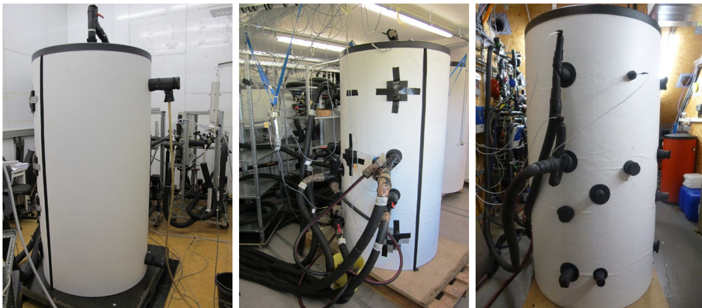
Figure 1: The Store installed at the testing laboratory igte, ise and SPF. Depending on test sequence different connectors are connected.
