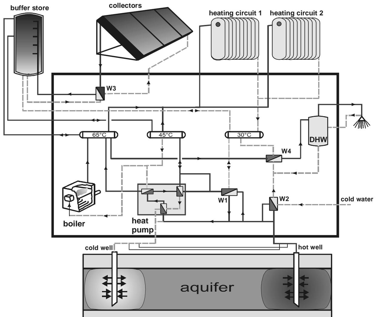
Figure 1: Scheme of the heat supply system (W1-W4: heat exchangers; DHW: domestic hot water)
