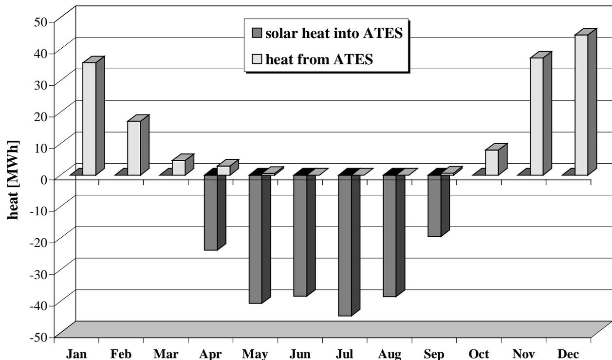
Figure 5: Monthly heat balance for the ATES
