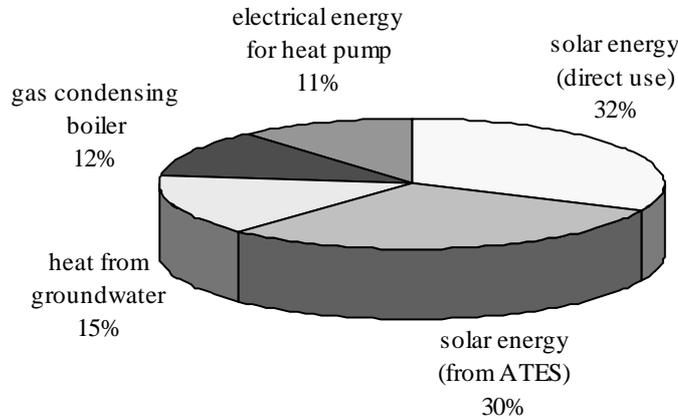
Figure 3: Relative contributions of the heat producers in the heat supply system
