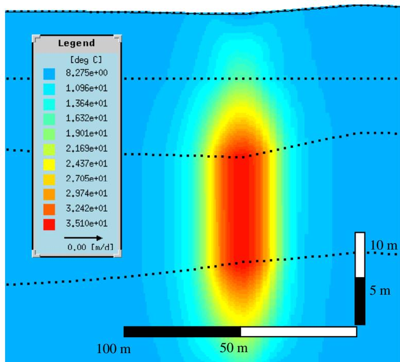
Figure 4: Temperatures in the warm bulb in the first year (vertical section)
