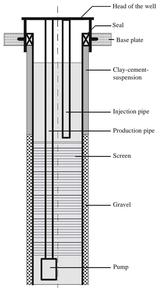
Figure 2: Construction of the wells
