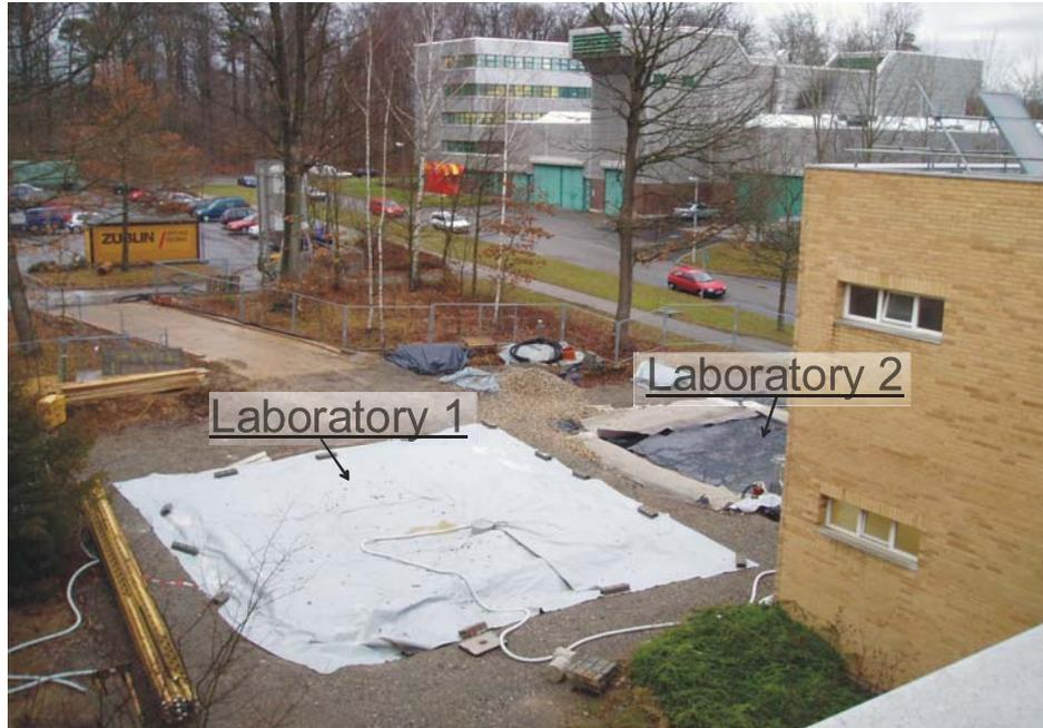
Figure 1: Field tests - the two outdoor laboratory-pit heat stores: left hot-water-pit heat store with floating cover, right gravel-water pit heat store, (cover not yet completed).
