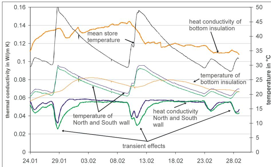
Figure 3: Trend of the thermal conductivity and the mean temperatures of the North and South wall as well as of the bottom insulation of laboratory 2.
