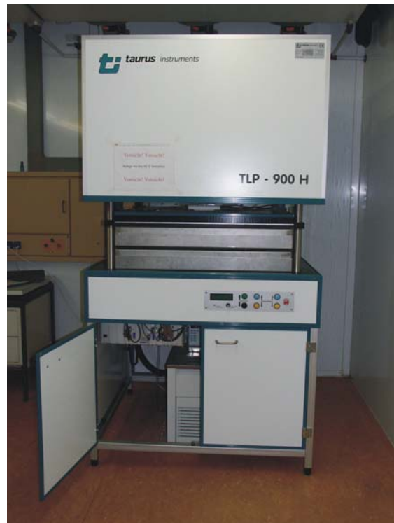
Figure 1: Protected heating plate with stainless steel bulk container
