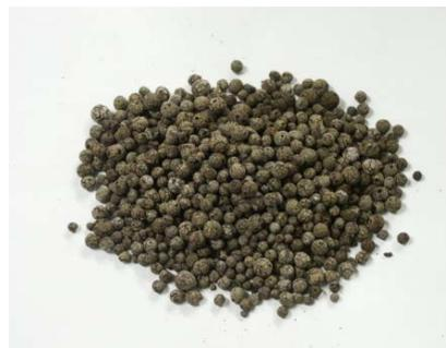
ECG,  $d = 4-8 \text{ mm}$ ,  $\rho = 270 \text{ kg/m}^3$
