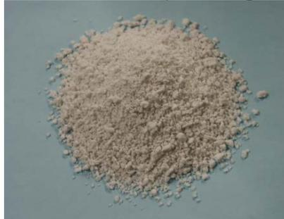
EP,  $d = 1 \text{ mm}$ ,  $\rho = 100 \text{ kg/m}^3$
