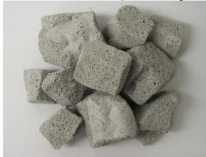
FGG,  $d = 10-50 \text{ mm}$ ,  $\rho = 170 \text{ kg/m}^3$
